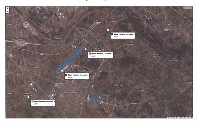
Two fixed measuring devices are close to the edges of runway 04 and 22. Distance of station NMT 1 from edge of runway 04 about 306 meters, distance of station NMT 2 from edge of runway 22 about 307 meters.
